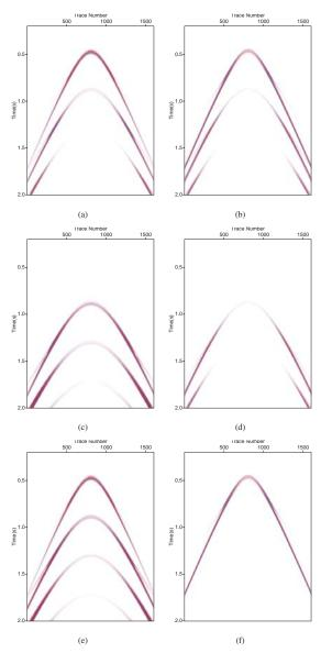
Figure 3: The left column is data and processing with ghosts in the data , and the right column is data and processing with ghosts removed. (a) and (b) are input data, (c) and (d) are free surface multiple predictions, and (e) and (f) after free surface multiple removal through a simple subtraction. Comparing (e) and (f) shows the residual if we do not remove ghosts.
