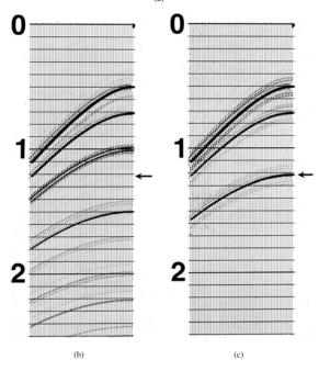
Figure 1: Hidden reflector example: (a) Synthetic Model; (b) Shot record; (c) Shot record after an accurate amplitude and phase prediction of free surface multiple elimination. This example shows that the ISS free surface algorithm doesn't require a residual Radon or adaptive step. Note that the energy minimization criteria fails in this example. (Example provided courtesy of Bill Dragoset.)
